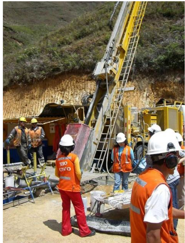
Core extraction at drill site
